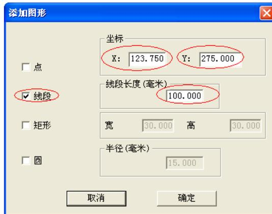
The screenshot shows the '添加图形' (Add Shape) dialog box. The '点' (Point) checkbox is unchecked. The '线段' (Line) checkbox is checked and circled in red. The '坐标' (Coordinates) section has 'X: 123.750' and 'Y: 275.000' both circled in red. The '线段长度' (Line Length) is 100.000, also circled in red. Other options like '矩形' (Rectangle) and '圆' (Circle) are unchecked. The '宽' (Width) is 30.000, '高' (Height) is 30.000, and '半径' (Radius) is 15.000. '取消' (Cancel) and '确定' (OK) buttons are at the bottom.
