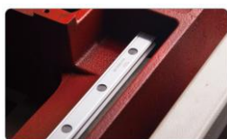
• 进口THK导轨 THK linear bearings
